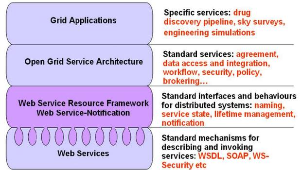
Fig. 1 The Open Grid Services Architecture., adapted from [8]
