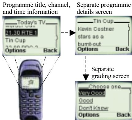
**Figure 6.** The WAP-PTV system adapts PTV for use on the new generation of WAP devices. The screen shots illustrate portions of a WAP-PTV guide.
