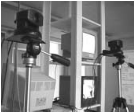
Figure 1: The ‘Talking Heads’ experimental setup with two steerable cameras capturing images of geometrical figures in front of them. Each camera is used by an agent in a grounded language game.
