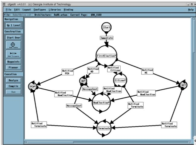
Figure 8. The Robot State Automata Diagram.
