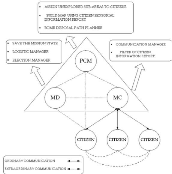
**Figure 3.** The MIP Architecture: A hybrid architecture with a dynamic and intelligent turnover of a government of three robots for the coordination of citizen, bomb-disposal executor robots.
