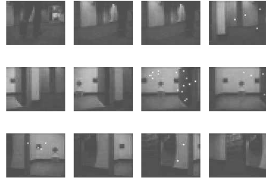
Figure 4. A behavior B has been learned, first consisting entering a small room. This figure shows a camera panoramic movement of a corridor and room entrance. The light pixels correspond to detected features of B . Their are more features detected in front of the room entrance, indicating when B can be applied. U_B(X) is reported in figure 5
